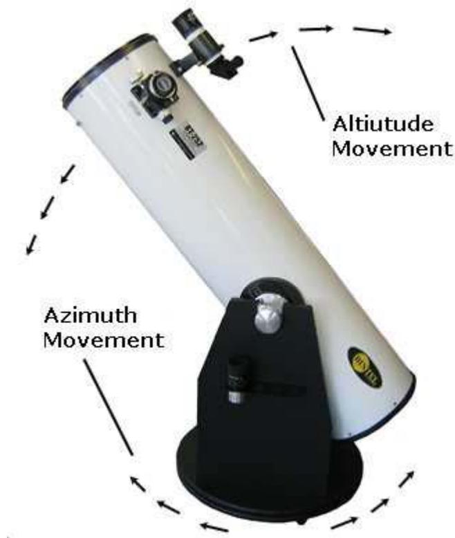
Move the telescope gently. You can adjust / tighten the side movement, from the side of the base. Please ensure it's adjusted to move smoothly, but not be loose or unstable.
