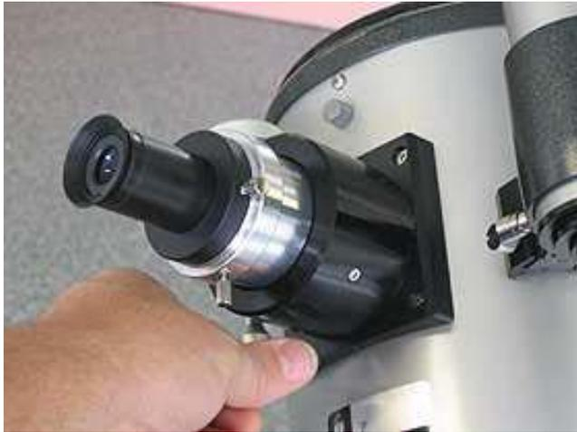
If you have trouble focusing, rotate the focusing knob so the drawtube is in as far as it will go. Now look through the eyepiece while slowly rotating the focusing knob in the opposite direction. You should soon see the point at which focus is reached. On the underside of the focuser there are two metal thumbscrews. The thumbscrew closest to the body of the scope will lock the focuser position; the other thumbscrew will adjust focuser tension.
